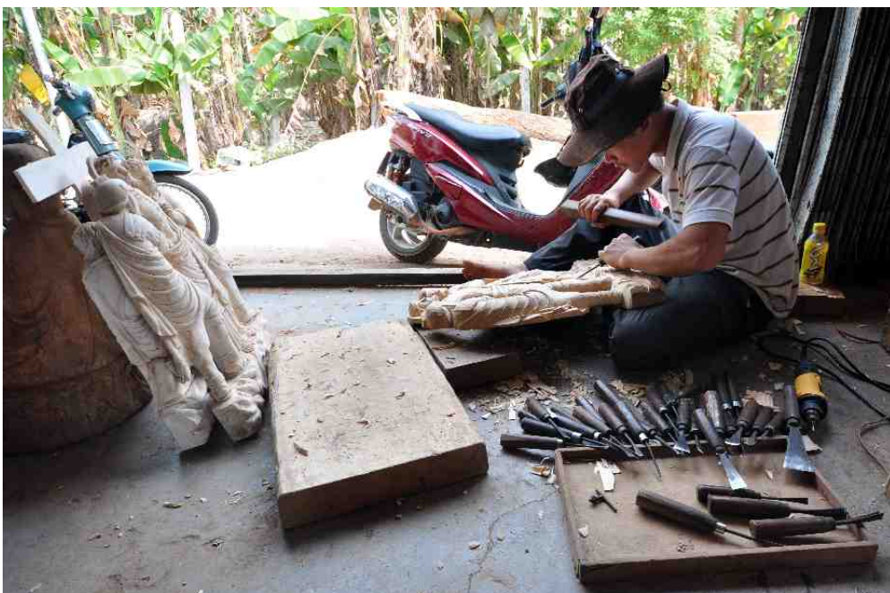
Hand carving a station of the cross, with the original template in front for comparison.
