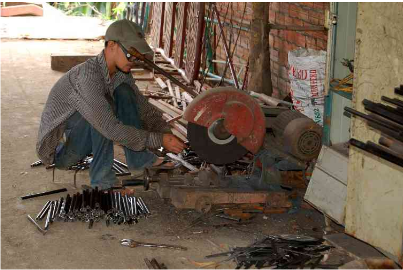
Cutting steel for chair components.
